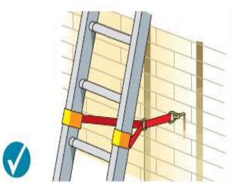
Tying near the base
