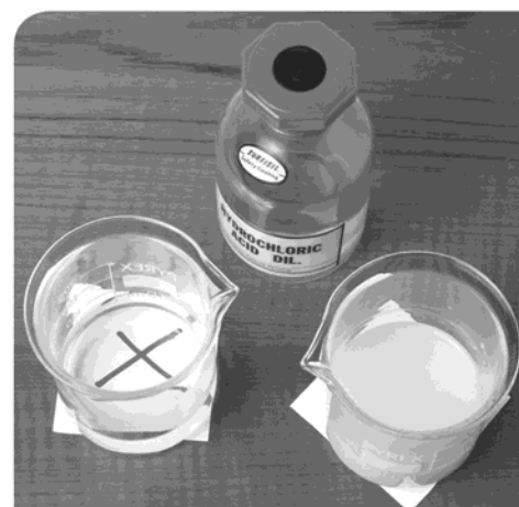
B We can follow the rate of the reaction between sodium thiosulfate and hydrochloric acid by measuring the time taken for a 'cross' drawn beneath the reaction beaker to disappear.
